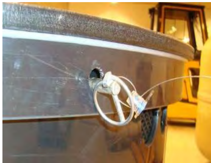
Picture 11 - Example of a sealed PhosClear unit
